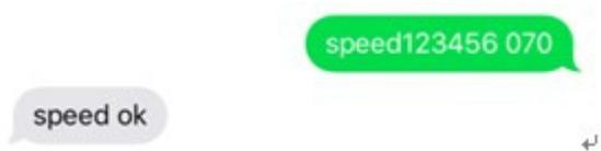
When the unit speed is over 70km/h, it will send message “speed alarm!” to the admin number every 5 minutes.
